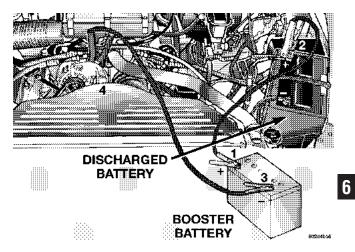
5. Connect the other cable, first to the negative terminal of the booster battery and then to the engine of the vehicle with the discharged battery. Make sure you have a good contact on the engine.
